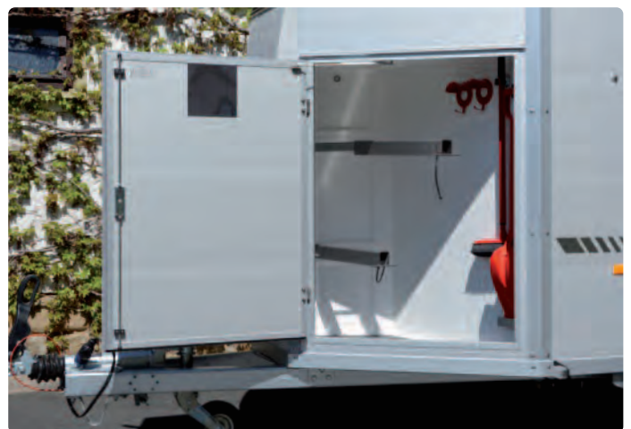
Sattelkammer Groß, Sattelhalter Saddle Supreme (ausziehbar) Grande sellerie, supports de selle Saddle Supreme (escamotables) Grand saddle chamber, Saddle Supreme saddle racks (slide-out system)
