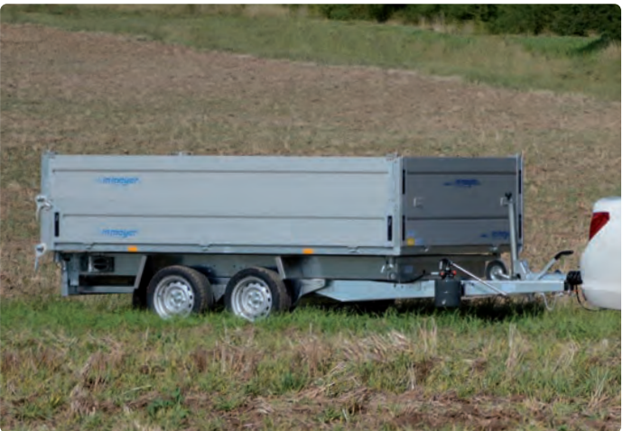
HKC 3031/186 Handpumpe, Zubehör: Alubordwanderhöhung HKC 3031/186 Pompe manuelle, option : ridelles supplémentaires en alu HKC 3031/186 Manual pump, option: additional aluminium side panels
